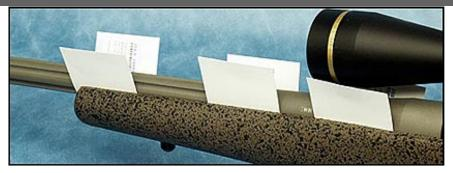
This full-floating barrel will remain perfectly centered in the barrel channel of this laid-up fiberglass stock. Were it a one-piece stock of walnut, the gap between metal and wood would probably change between seasons or if subjected to a drenching.
