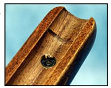
Most production rifles with onepiece wood stocks are factory bedded using a pressure "band" at the fore-end tip; it's the only contact between forearm and barrel. It can either be filed away to float the barrel or shimmed to apply more pressure.
