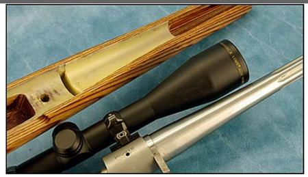
The author generally floats the thin portion of the barrel starting where the straight taper to the muzzle begins. On this particular rifle he then had a mortise milled into the bottom of the remaining barrel channel to lighten the stock.
