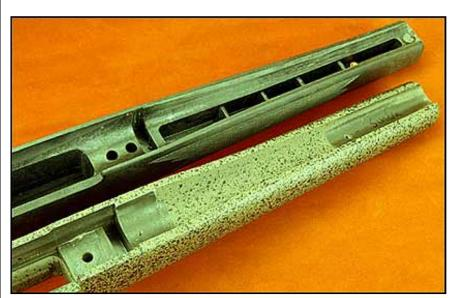
Injection-molded stocks are unsuitable for glass bedding and generally have hollow fore-ends that further preclude the process. Note the small, circular pressure pad at the tip. Laid-up stocks take to glass bedding well.
