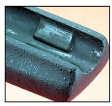
Remington's new Model 700 Light Varmint rifle has a laid-up fiberglass stock with a unique tip arrangement whereby two pads on either side of the barrel channel apply dampening pressure while also centering the barrel as would a V-block.
